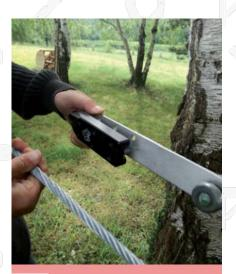
Place the cable and te Matrix on the plate.
