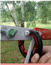
The final tightening torque will be made after a few passes on the cable. This operation is to be reproduced for all packs. Check that the hook slides on the plate.
